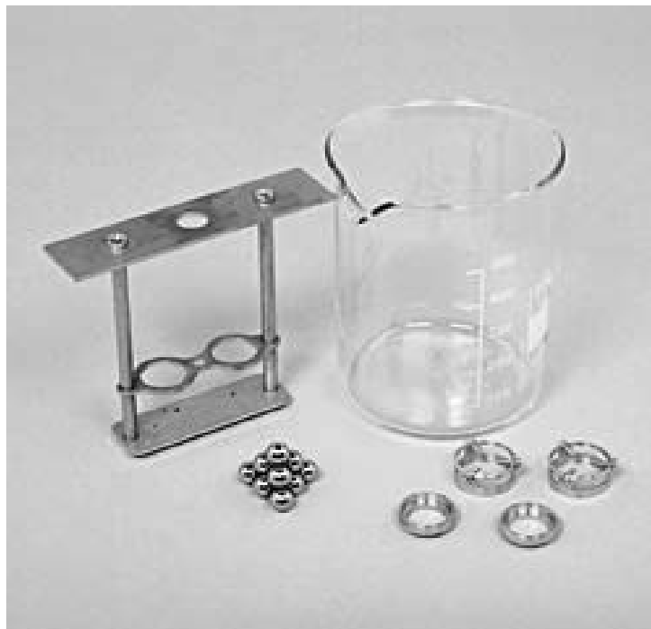
Figure 2: Softening Point Test Apparatus accessories
