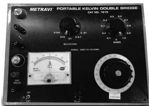
Figure 1 Front view of Kelvin Double Bridge
