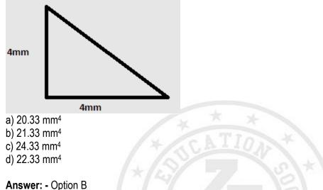
**Explanation:** - The moment of inertia of a triangular section about the base =  $bh^{3}/12$ . = 4x4x4x4/12
