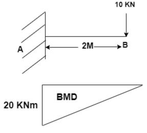
62. Which of the following statements are correct about a cantilevered beam with point load acting on the extreme end of the beam?
