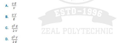
**Answer: -** Option D **Explanation: -** Strain Energy=1/2\*LOAD\*DIPLACEMENT=σ<sup>2\*</sup>Vol<sup>m</sup>/2E.
