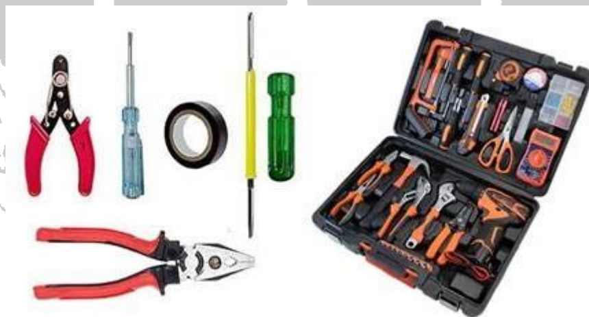
Fig. 4.1 Tool Kit and Electrical Technicians Main Tools
