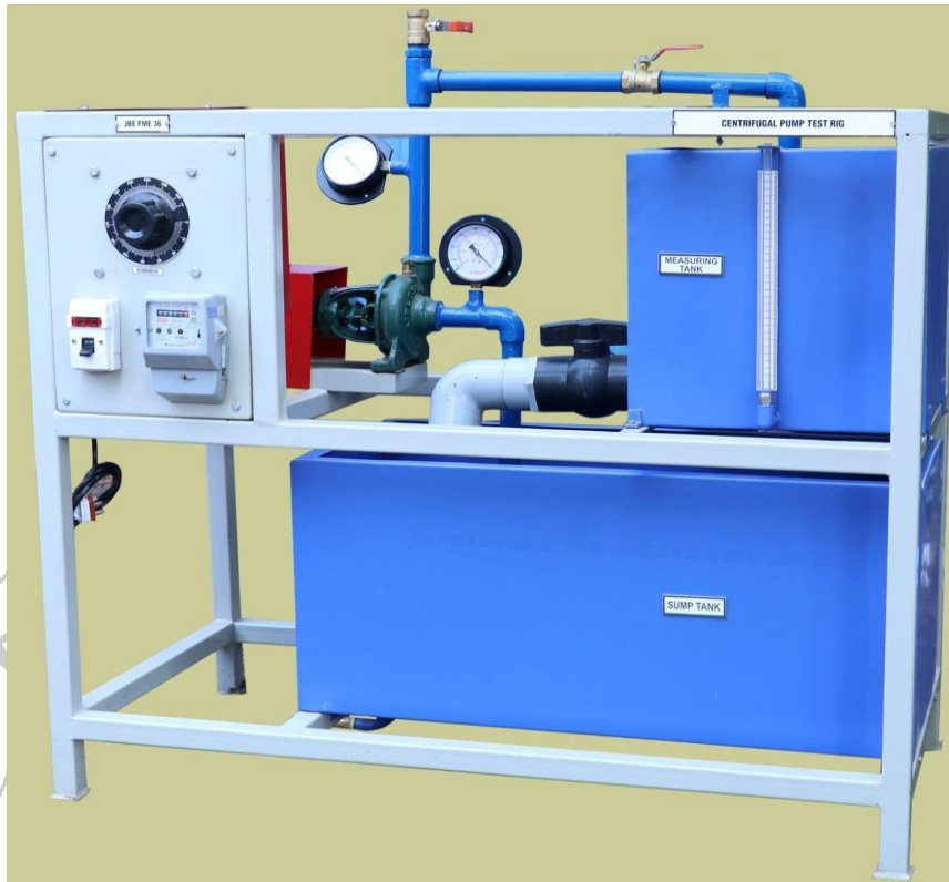
Figure 14.1- Centrifugal Pump Test Rig
