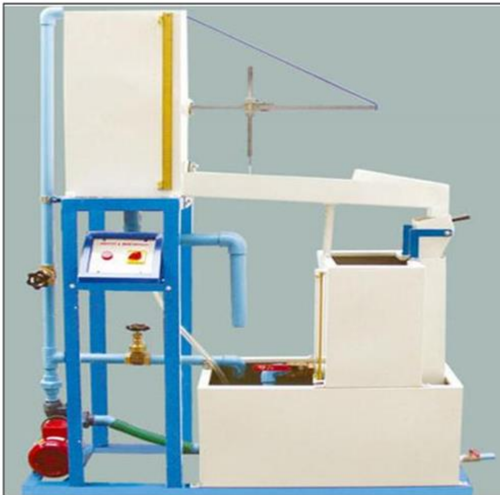
Figure 5.3 Experimental set up of measurement of discharge through a pipe provided with sharp edge circular orifice
