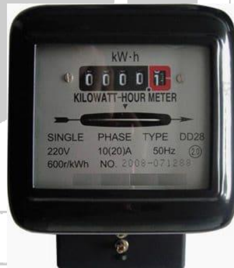
Figure 1.4 Single phase Energy Meter (Mechanical)
