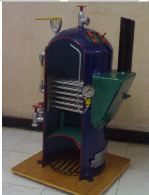
Fig 3.2 Cut section model of Cochran Boiler
