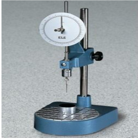
Figure 4.1: Bitumen Penetrometer & Concept of penetration resistance of bitumen
