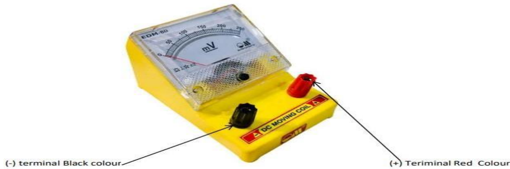
Fig:1.2 Terminal markings on Moving Coil (MC) instruments
