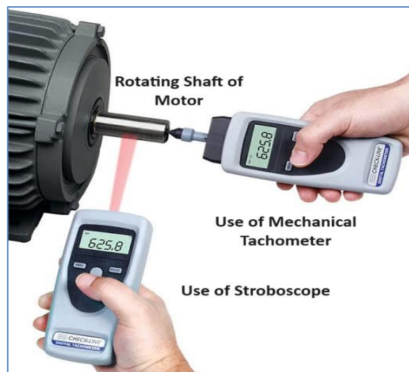
Fig. 3 Experimental set up of speed measurement by Stroboscope & Analog Tachometer.
