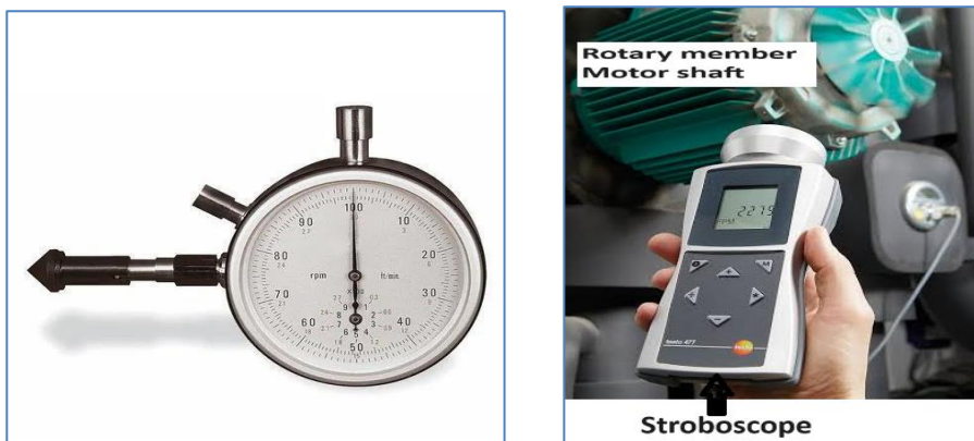
Fig.2 Mechanical Tachometer (Analog Tachometer) and use of stroboscope
