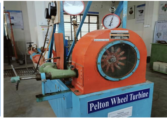
Fig.3 Pelton wheel turbine sketch and set up
