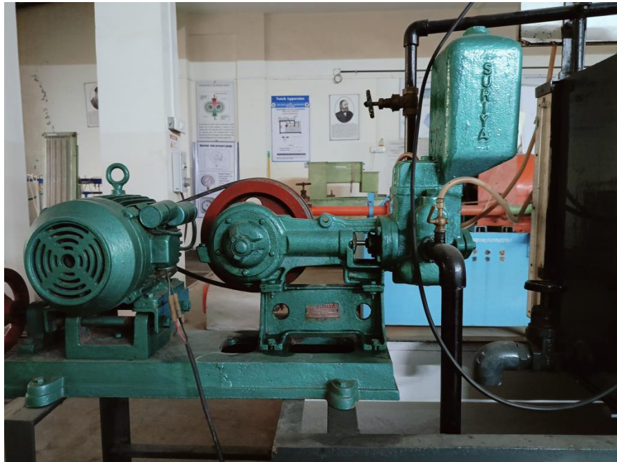
Fig.2 Set up of Reciprocation pump
