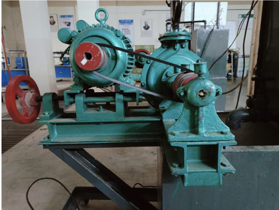
Fig.2 Setup of Centrifugal pump
