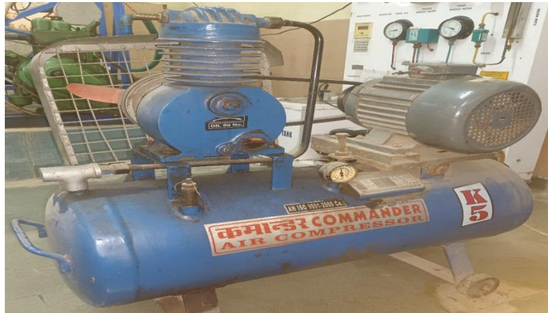
Fig. 4 Laboratory Equipment – Single Stage Air Compressor
