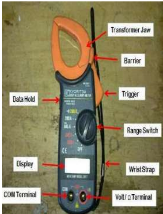
Fig 1 Front View of Clip on Meter
