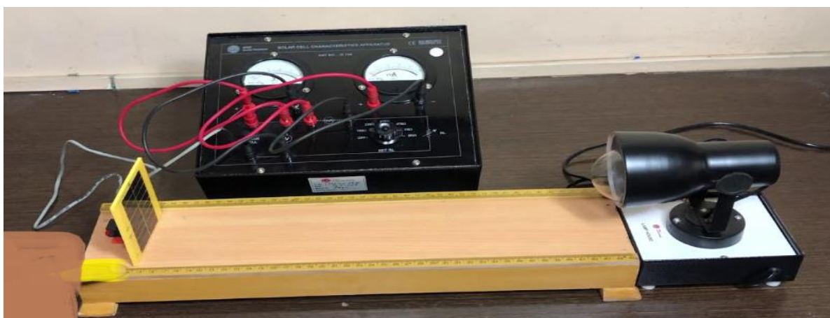
Figure 14.4 Experimental Set-up for Solar Cell Characteristics
