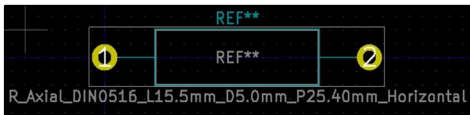
Figure 12.14 An example of a footprint for a resistor. The yellow circles represent holes.
