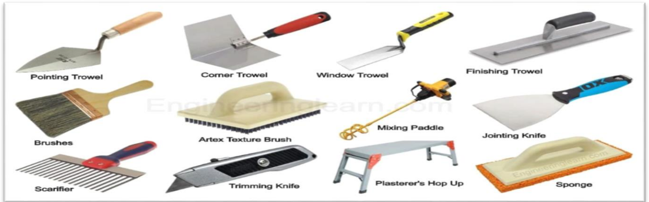
Figure 16.2: Tools for plastering and Pointing
