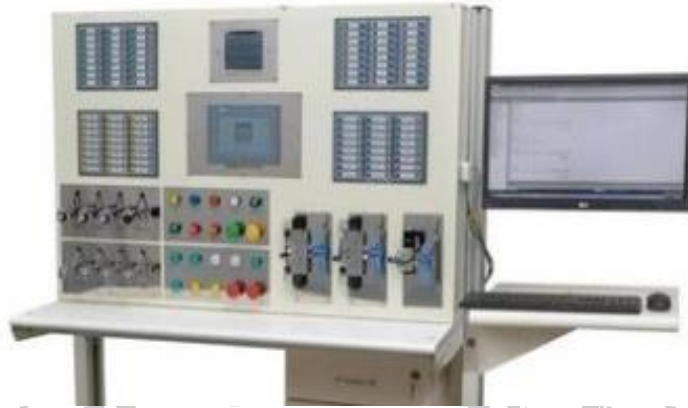
Fig. 2.1: A photograph of PLC trainer kit
