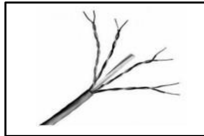
Fig. No. 4.5. Separate pair wires
