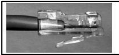
Fig.No.5.7. Fit cable in to Connector
