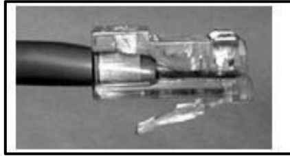
Fig. No.4.7. Fit cable in to Connector
