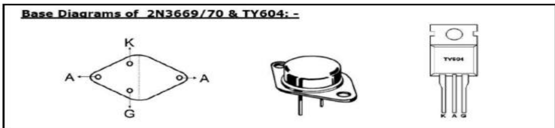
Fig. 1.3 Base Diagrams of SCR 2N3669/70 & TY604
